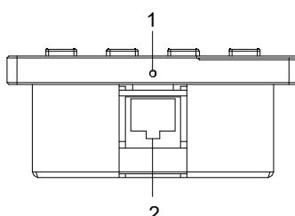
1. Bottom Box Fixing Screw Hole
