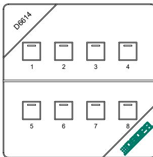
As can be seen from the above figure, the panel is composed of 8 buttons, each button has an indicator light, the indicator light is on when pressed, and different commands can be programmed for the 8 buttons according to the needs, and the corresponding commands can be remotely controlled by pressing the buttons.
