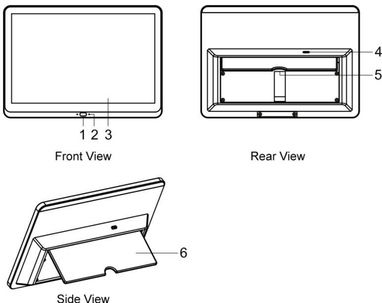
1. Power Button: Press and hold the button to power on, power off or restart. Press the button once to turn on/off the screen.
